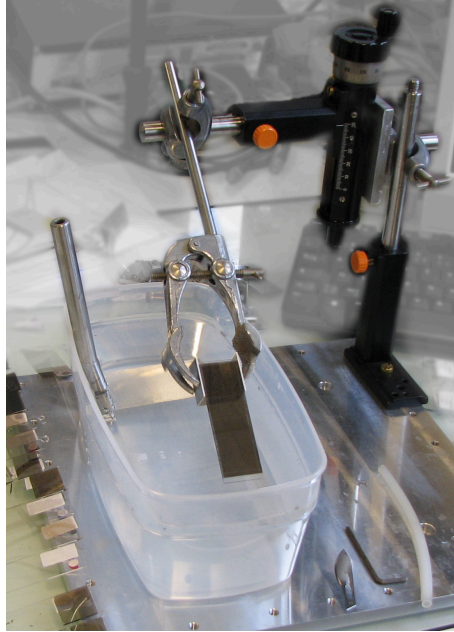
Figure 5.4: The simple but practical setup for preparing the nanofoils onto a frame. The procedure is described in the text. It requires a great deal of practice and patience to obtain very flat foils as shown on the right photo in figure 5.3.
